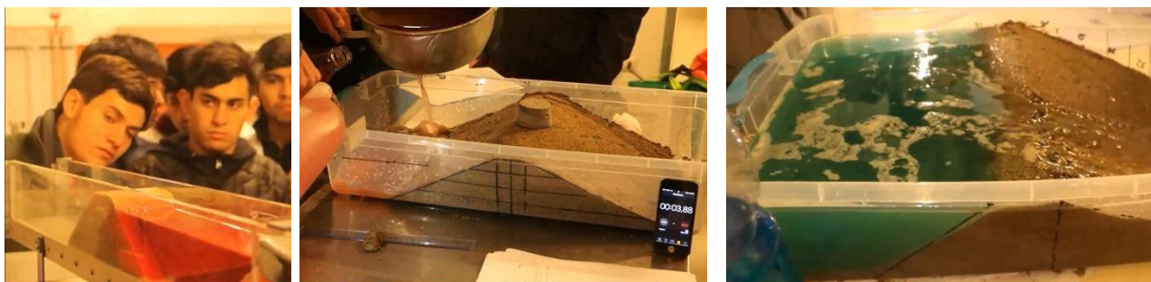
a) Observing water seepage b) Soil dam is charged with water-running video/clock c) Water and soil behavior during overtopping
